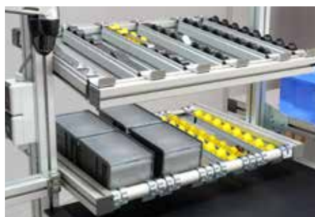
The flexible roller carrier system enables a particularly variable solution for kanban.
