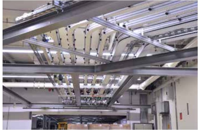
A large part of the conveyor system was installed under the ceiling at a height of three to five metres.
