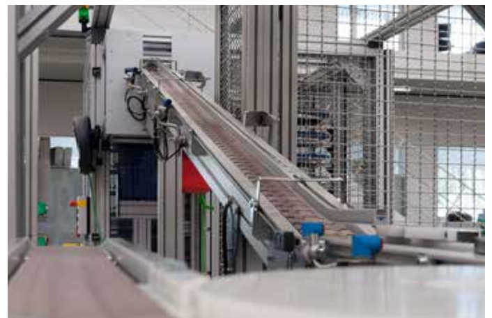
Segmented chain conveyors are particularly suitable for large and complex system.
