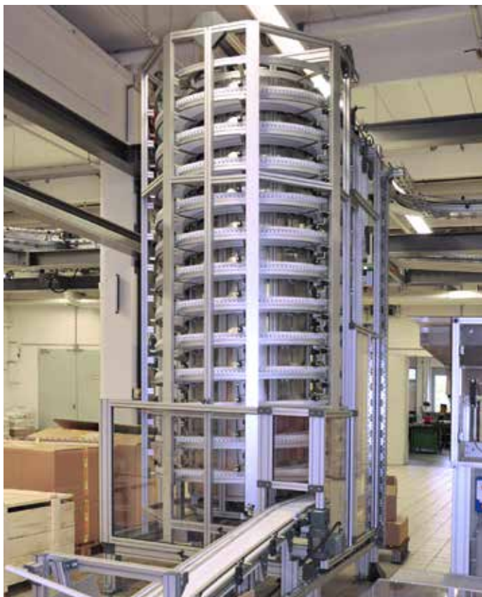
The nine storage towers, each with a 50 metre conveyor section, ensure constant material flow even at full load.
