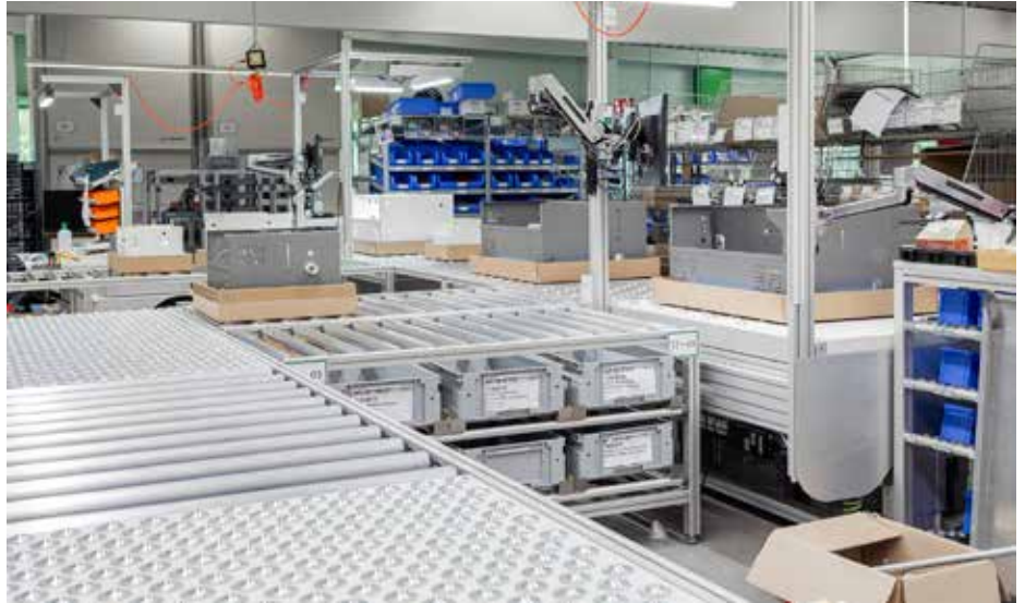
Roller conveyors and ball transfer tables for transporting workpieces between the workstations.
