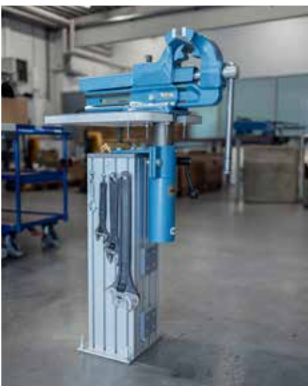
Special solution: height-adjustable vice.
